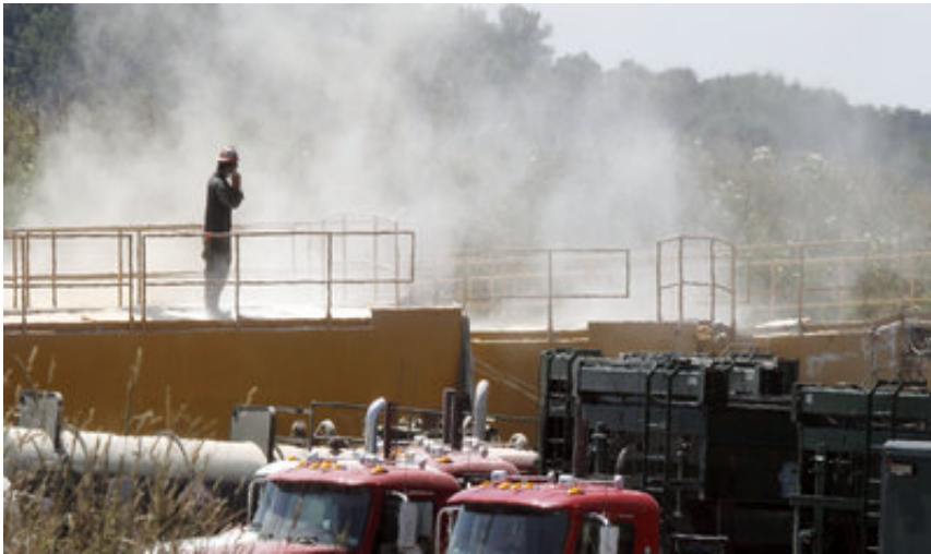
Figure 18: Fine fracking silica sand particles are a threat to workers. Source: http://media.npr.org
