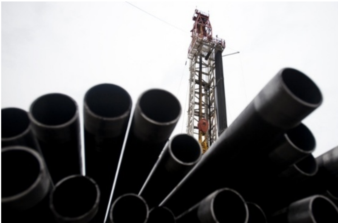
Figure 9: Fracking well pipes stacked at fracking site ready for assembly and submersion into the ground.
