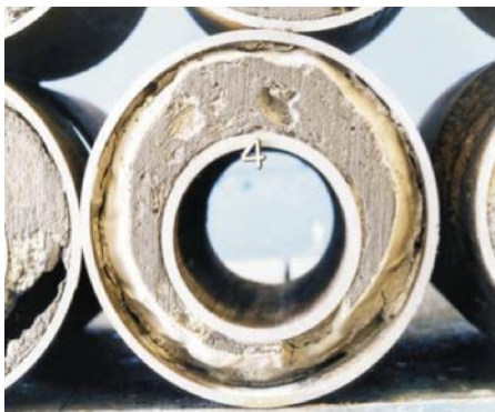
Figure 10B: In reality, the concentricity of pipe cemented casing, particularly once the wellbore begins to migrate horizontally—sending the internal casings to the bottom due to gravity, is more likely to be like in this image, where there is more manifest eccentricity , than concentricity. That is, the internal piping pushes downward, leaving a dangerously thin layer of cement separating the pipes. In this image we also see the contamination of cement by drilling mud, causing weaknesses in the cement integrity which can also lead to contamination. Source: Desseault et.al.
