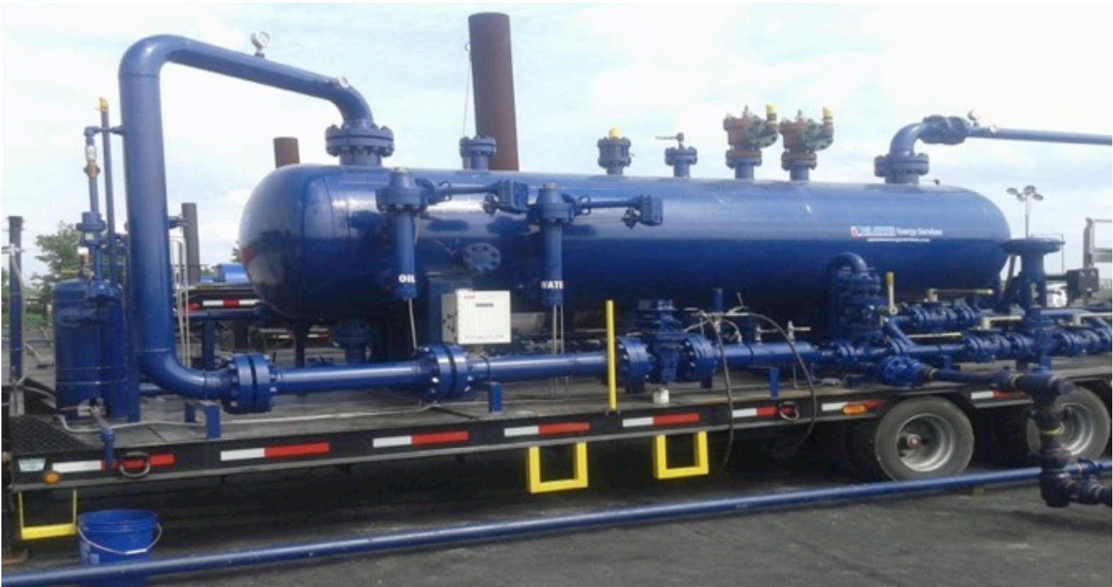
Figure 6: Tanks receive flowback water from a fracking well and separate water, gas, sand and oil. Photo: JDTaillant
