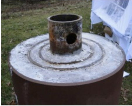
Figure 10A: Cemented concentric steel pipe used in fracking wells. This is an ideal design, since in practice the pipes (due to irregular positioning in the geology) may not be located in a concentric manner thereby thinning cement and reducing safety
