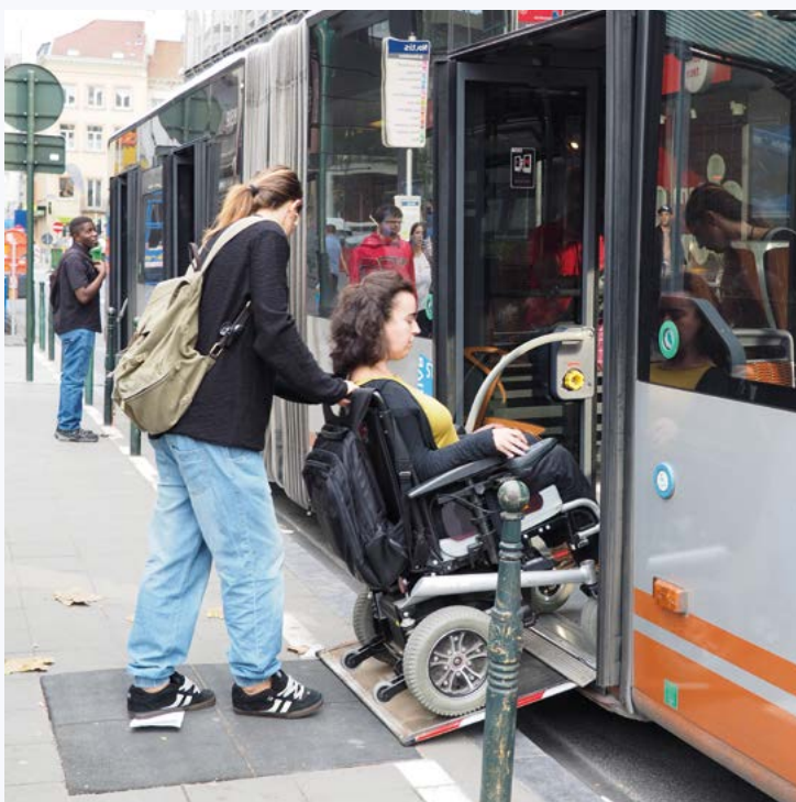
Low floor buses improve access to public transportation for the general public, particularly senior citizens and persons with disabilities, including those using wheelchairs and walkers. ©CBM/Benjamin Dard
