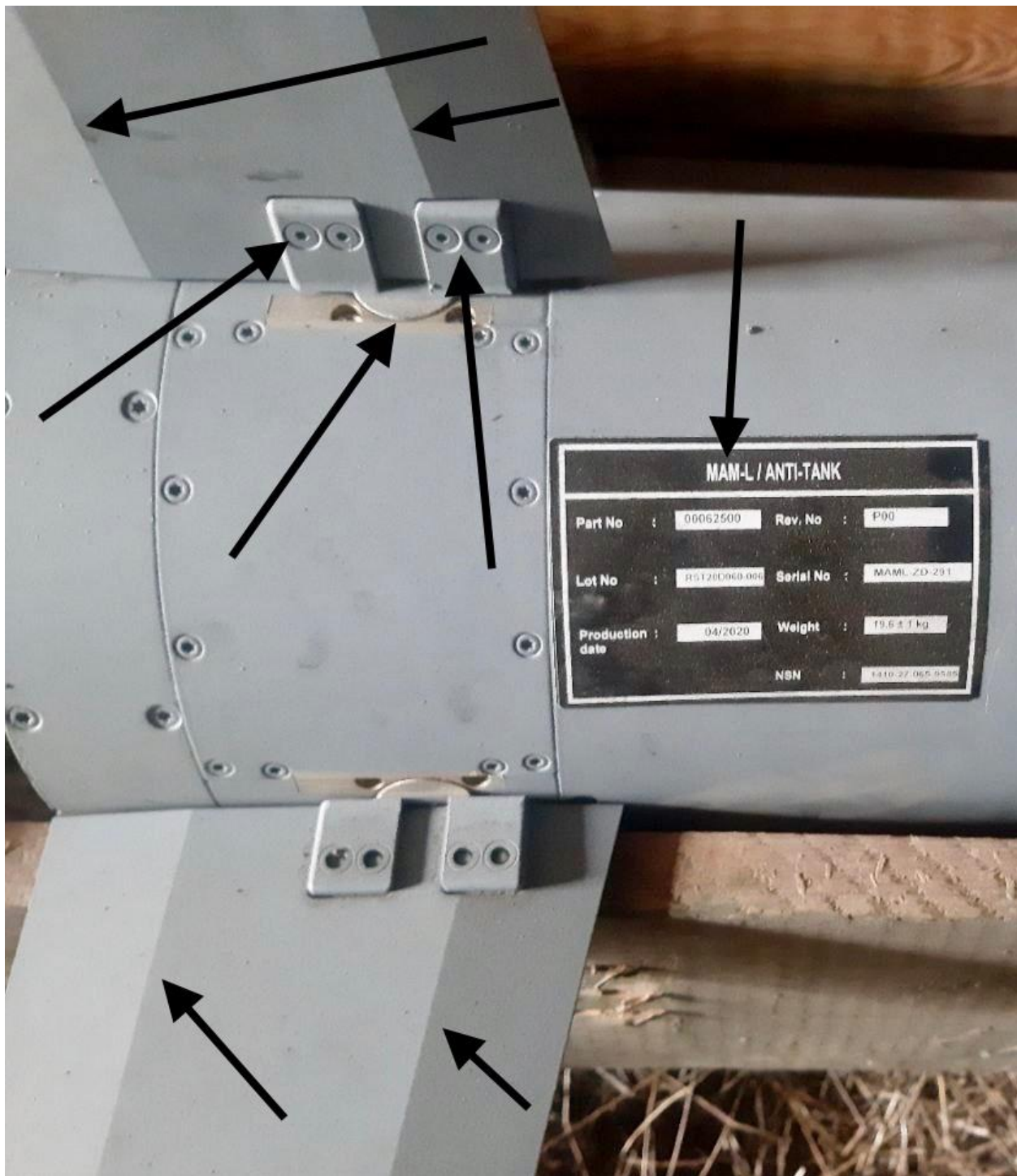
Image 3 : Close-up of tail section of a MAM-L bomb, highlighting tail fins' distinctive twin rectangular brackets with four-bolt pattern and circular attachment points to the fuselage. Image also shows distinctive ridge lines on the fins.
