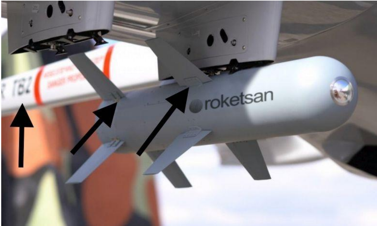
Image 1 : MAM-L smart micro munition (laser-guided bomb), manufactured by Roketsan, attached to a Bayraktar TB2 armed drone.
